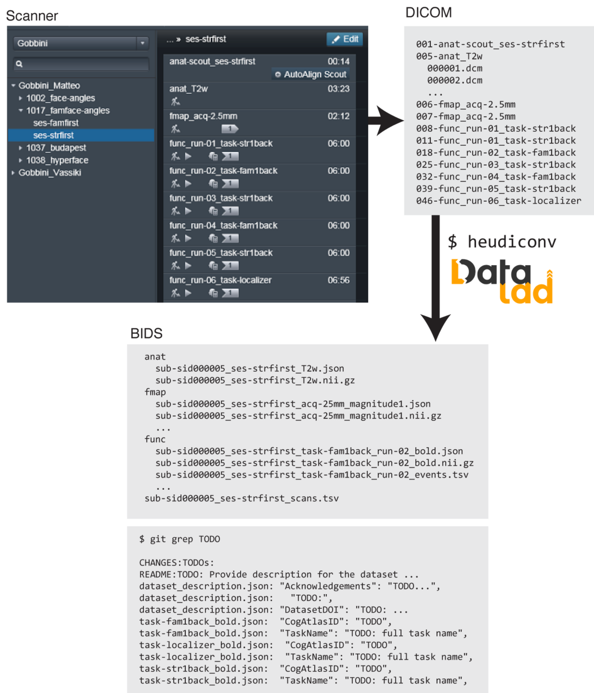
Figure 2. Example of the naming scheme at the scanner console, the resulting DICOM folder structure, and the automatically converted BIDS dataset. The user can quickly find what needs to be added by executing a simple git grep TODO , since the entire dataset is under git and DataLad control.
